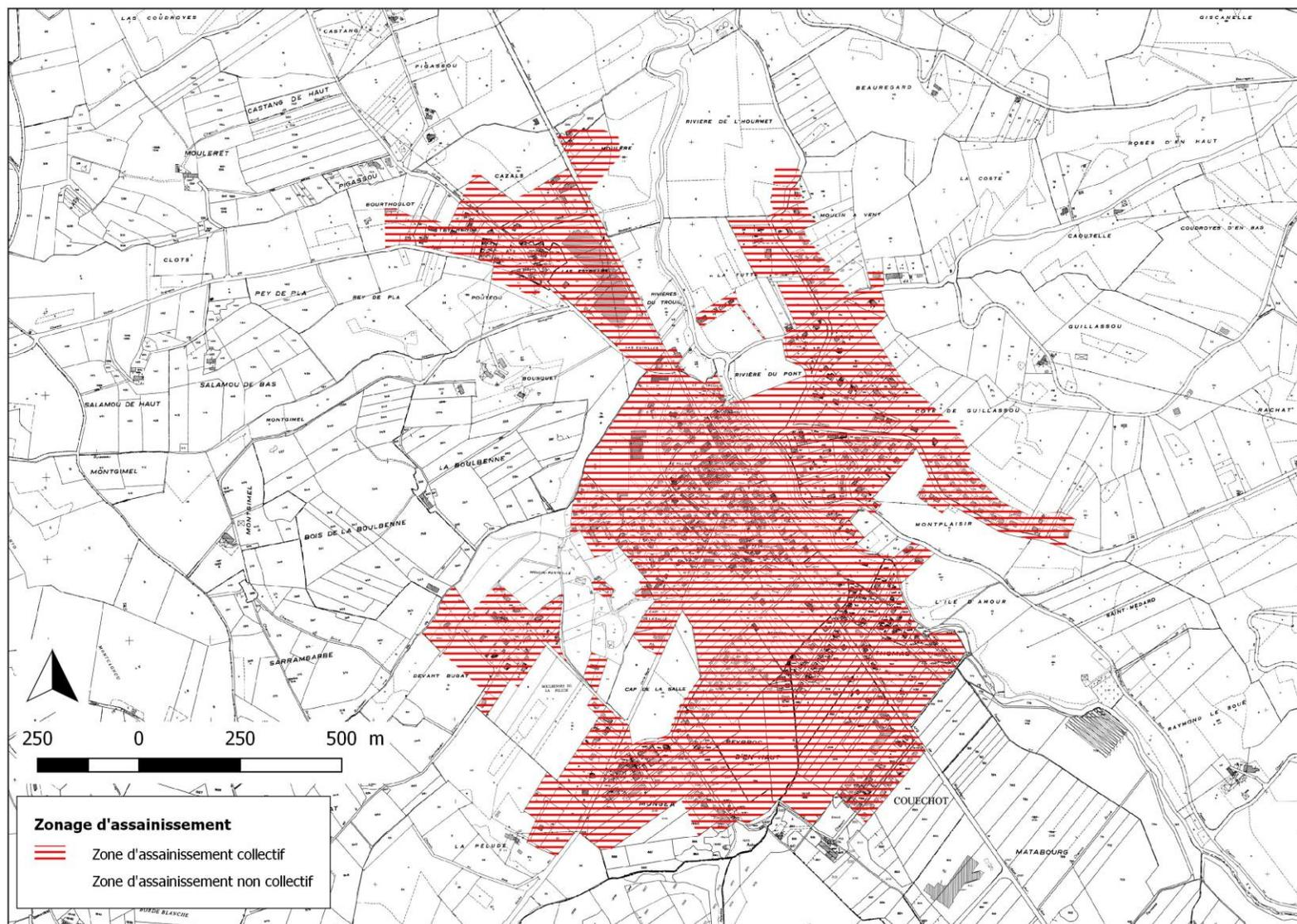
**FIGURE 10 : ZONAGE D'ASSAINISSEMENT PROPOSE**
