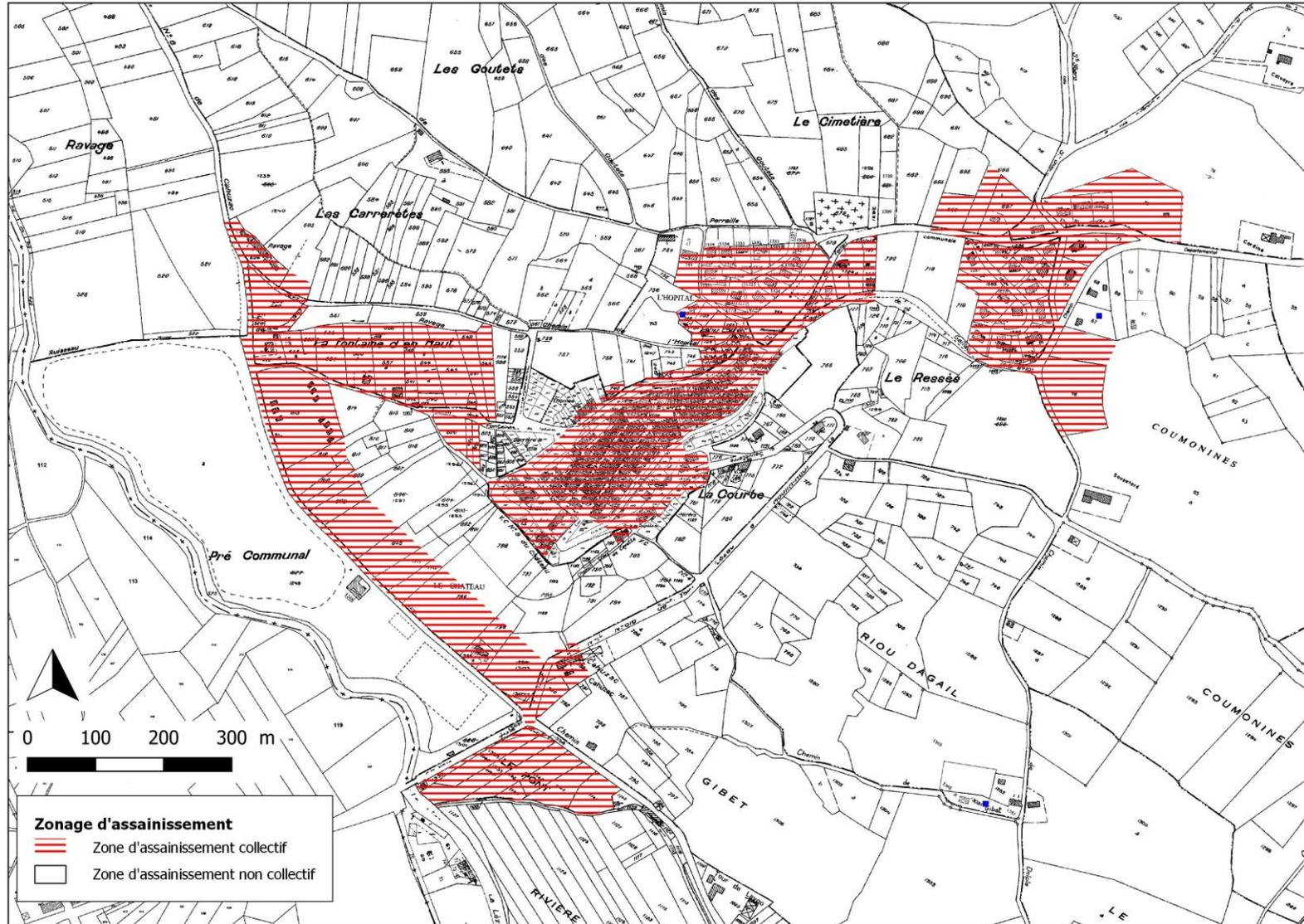
**FIGURE 11 : ZONAGE D'ASSAINISSEMENT PROPOSE**
